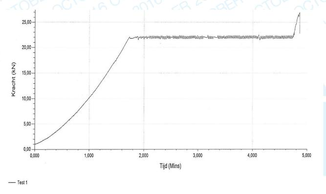
Figure 2 – Dynamic performance test: Graph of arrest force vs. time
